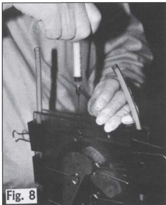
Fig. 8: BD Spinal needle being used to extract bubbles from cast specimen prior to curing.
