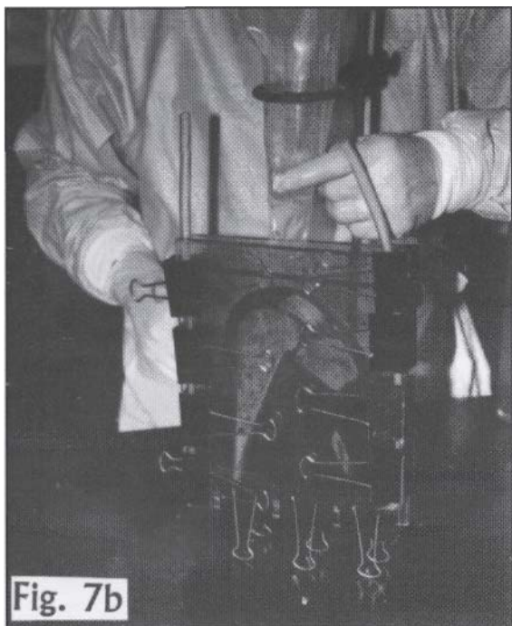
Fig. 7b: Filling funnel being used to fill specimen cast during embedding.
