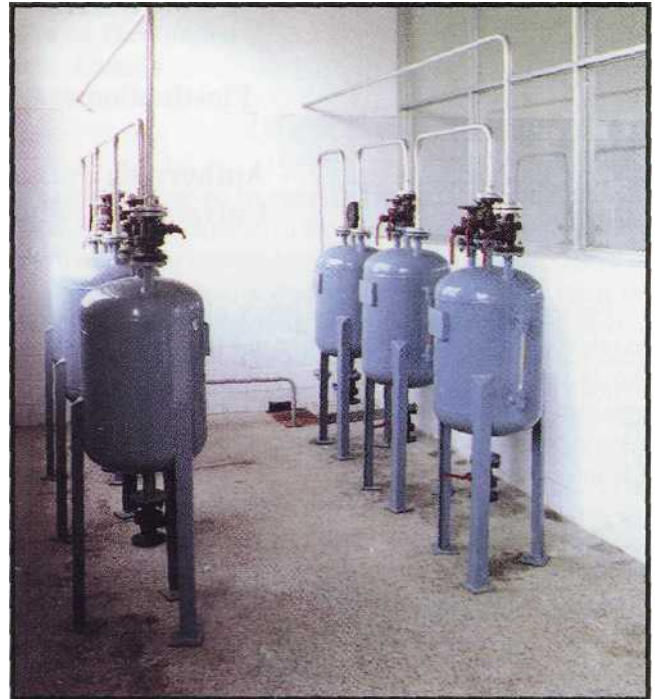
Figure 3. Stainless containers located between the vacuum chambers and the pumps to collect acetone vapors.
