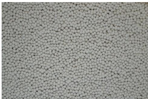
Figure 1: Molecular sieves with 3 Å pore.
