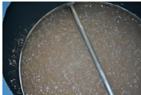
Figure 6: Reaction of acetone and sieves [boiling acetone (exothermic reaction)].
