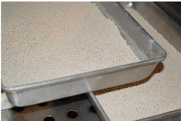
Figure 7: Molecular sieves in oven-safe metal container.
