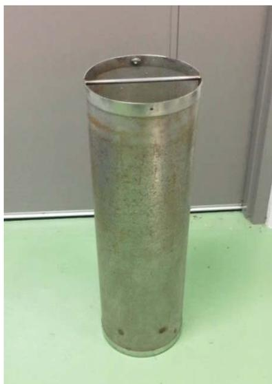
Figure 2: Perforated stainless-steel cylinder manufactured to house the molecular sieves
