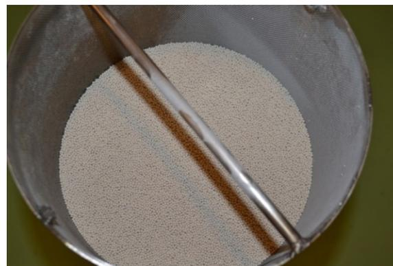
Figure 4: Molecular sieves inside the cylinder
