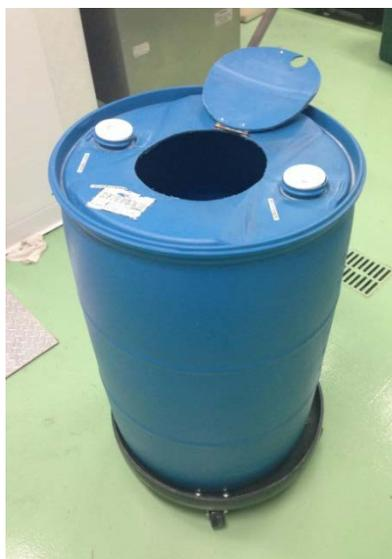
Figure 3: Modified 208 L (55 gallon ) plastic drum with 24.4 cm (10 inch ) diameter hole.
