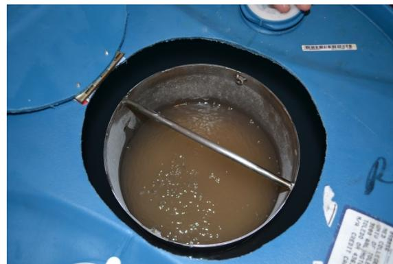
Figure 5: Modified 208 L (55 gallon ) plastic drum of acetone containing the stainless steel cylinder with the molecular sieves.
