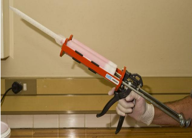
Figure 1. Silicone handgun with twin chamber cartridge loaded with red pigmented silicone.
