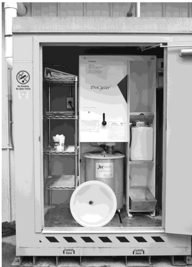
Figure 2. B/R Instruments Solvent recycler, in an explosion-proof enclosure.
