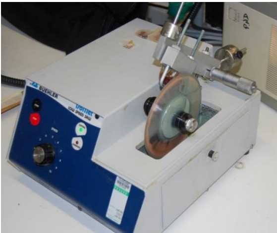
Figure 5. Sections were cut with a Buehler Isomet slow-speed diamond saw. The speed setting was set to 3.0.
