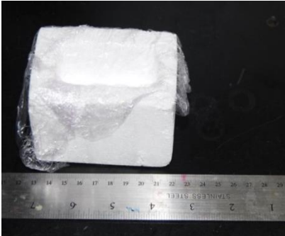
Figure 4. Molds were cut from blocks of Styrofoam and lined with plastic foil.
