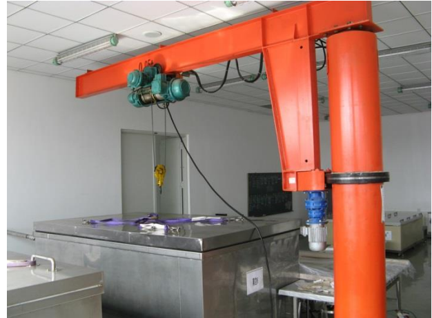
Figure 1 - A specially-designed bath and cantilever hoist were used for forced impregnation.
