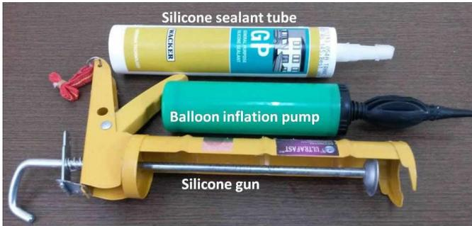
Figure 1: The balloon inflation pump, silicone gun, and silicone sealant tube before the infiltration procedure.
