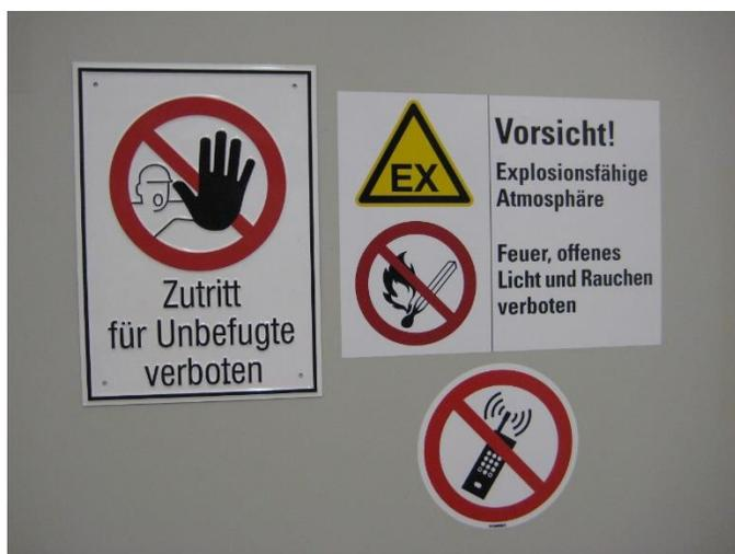
**Fig. 10: Prohibition signs at the entrance to a solvent storage. The yellow-black warning sign indicates the potential explosion hazard.**
