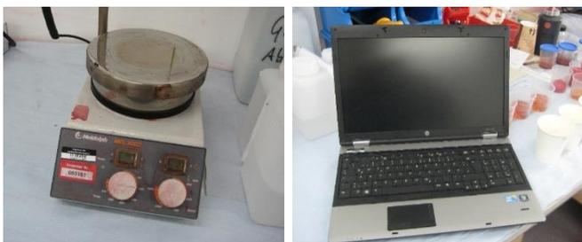
**Fig. 5: Electrical devices as potential ignition sources (examples): Magnetic stirrer with a heating plate, Computer.**
