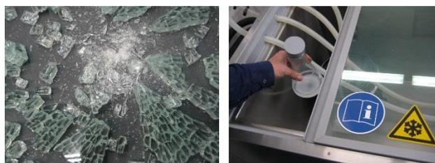
**Figure 2. Physical hazards: when damaged, a safety glass plate shatters into numerous small pieces (left). Working in the cold with unprotected hands bears the risk of cryogenic burns (right).**
