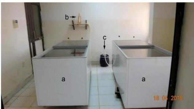
**Figure 1: Plastination laboratory set-up, showing: freezers (a) Bennert manometer (b) and separator (c).**
