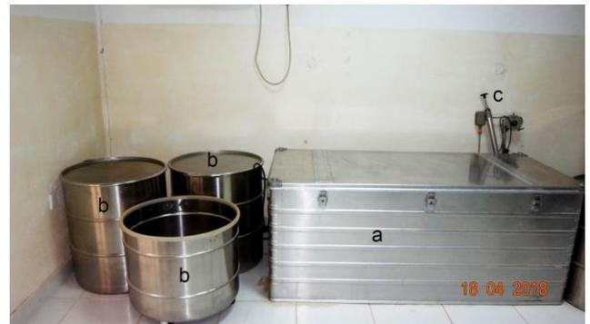
**Figure 2: Plastination laboratory set-up, showing gas curing unit (a); stainless steel drums (b) and conveyor pump (c).**
