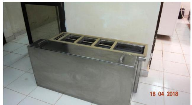
**Figure 3: Plastination laboratory set-up, showing dehydration and impregnation containers.**
