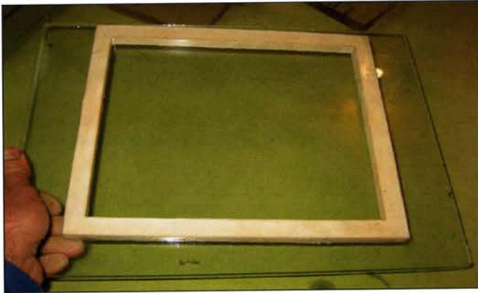
Figure 4. The increased weight, flexibility and smoothness of the silicon gasket prevents the formation of micropores between the gasket and glass.
