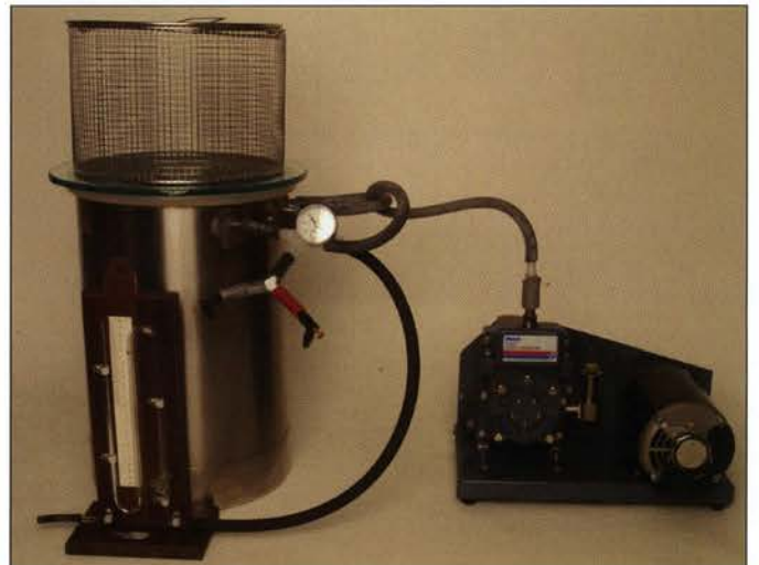
Figure 11. Impregnation setup. Vacuum kettle with basket, gauge and needle valves; vacuum pump; Bennert manometer.
