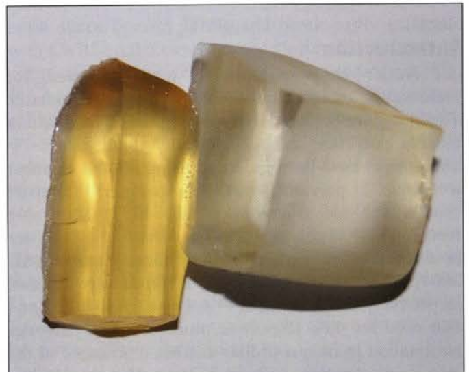
Figure 3. Comparison of cured block of early generation epoxy (left) and cured block of EP73 (right) six years post-curing.
