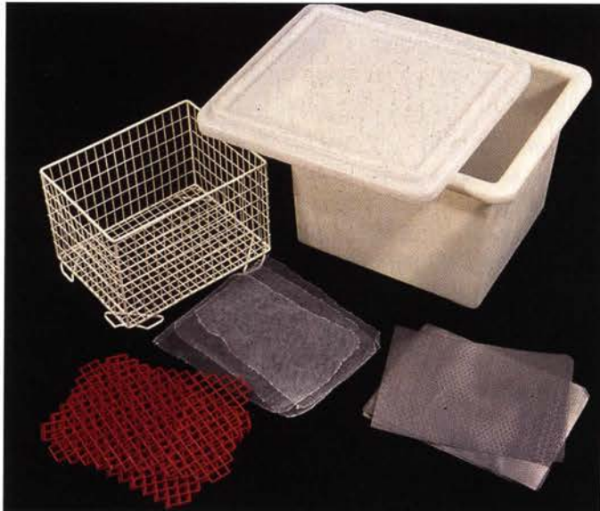
Figure 2. Accessories needed for stacking and bundling slices: Fly screen (f), grids - metal (m) and plastic (p), basket and reservoir.
