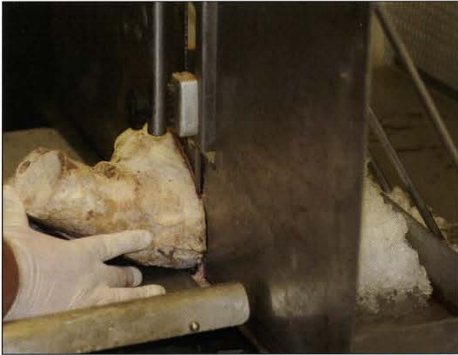
Figure 1. Slicing frozen tissue block on a band saw.
