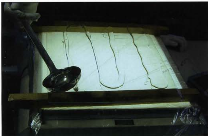
Figure 9. Sandwich curing technique: Casting-mixture poured onto heavy foil overlying the glass plate in preparation for impregnated slice.
