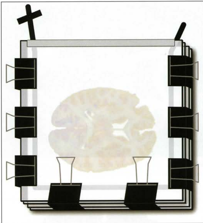
Figure 10. Flat chamber assembled, containing an impregnated slice, ready to be filled with resin-mix.
