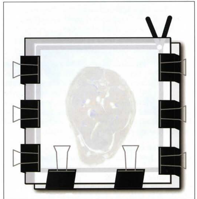
Figure 10. Sealed flat chamber ready for horizontal positioning and UVA light curing as the catalyst.
