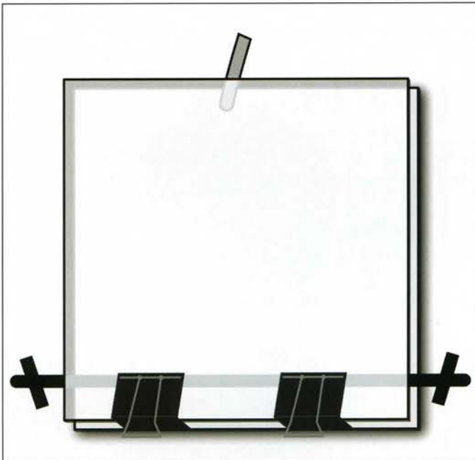
Figure 12. Building chamber for later insertion of the slice: Positioning top glass.
