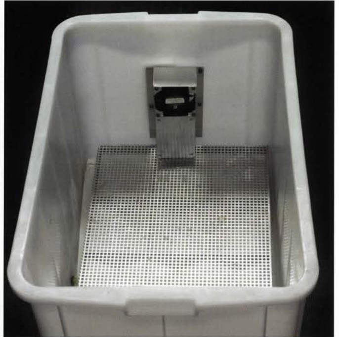
Figure 15. Curing chamber with spark-proof ventilator.
