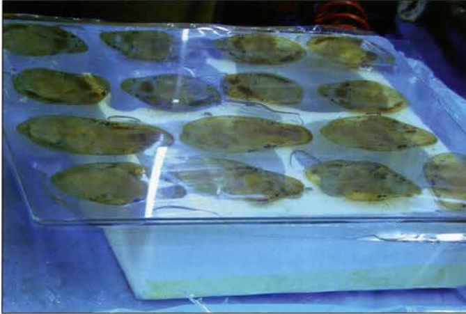
Figure 13. Sandwich curing technique: Glass is placed over foil.
