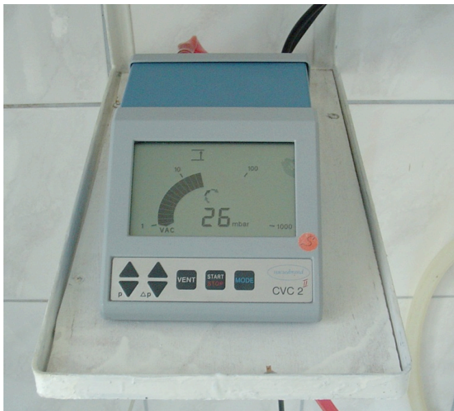
Figure 3. Digital controller for precise pressure control.
