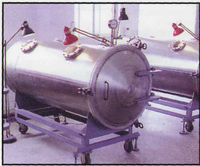
Figure 2. The mobile vacuum chambers.
