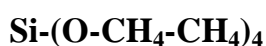
Figure 2. Structure of ethyl silicate. Si - refers to the silicone nucleus, which is covalently linked to four ethoxy groups.
