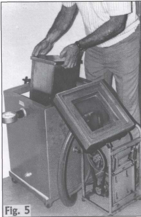
Fig. 5: Large vacuum oven placed on end being used as infiltration chamber. Size required is dependent upon size of plastination chamber used.
